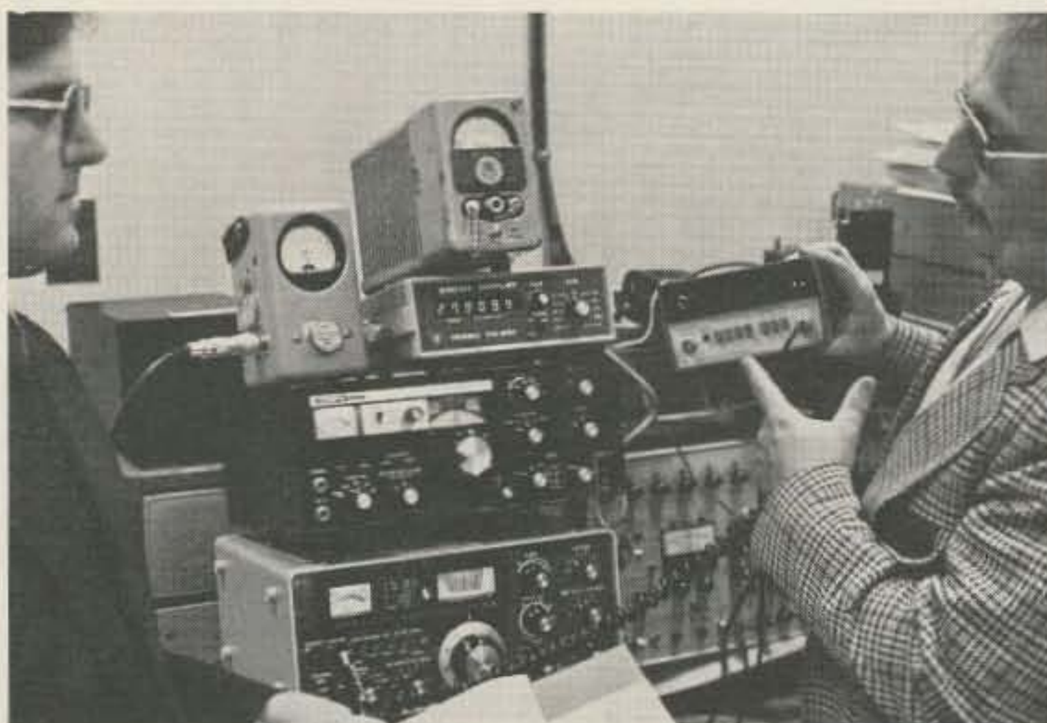
Some of the gear undergoing testing; note power output of 80 Watts and frequency of 27.9099 MHz.
