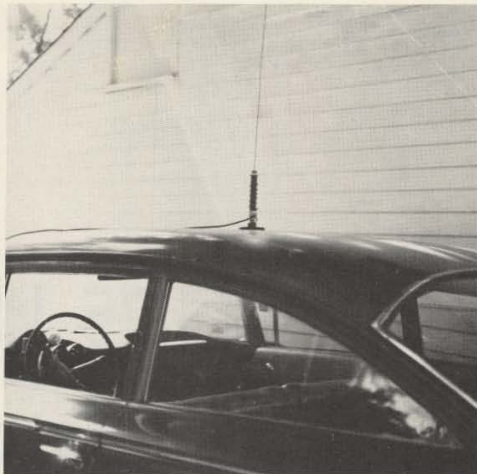
Antenna mounted on top of author's 1960 Chevrolet.
