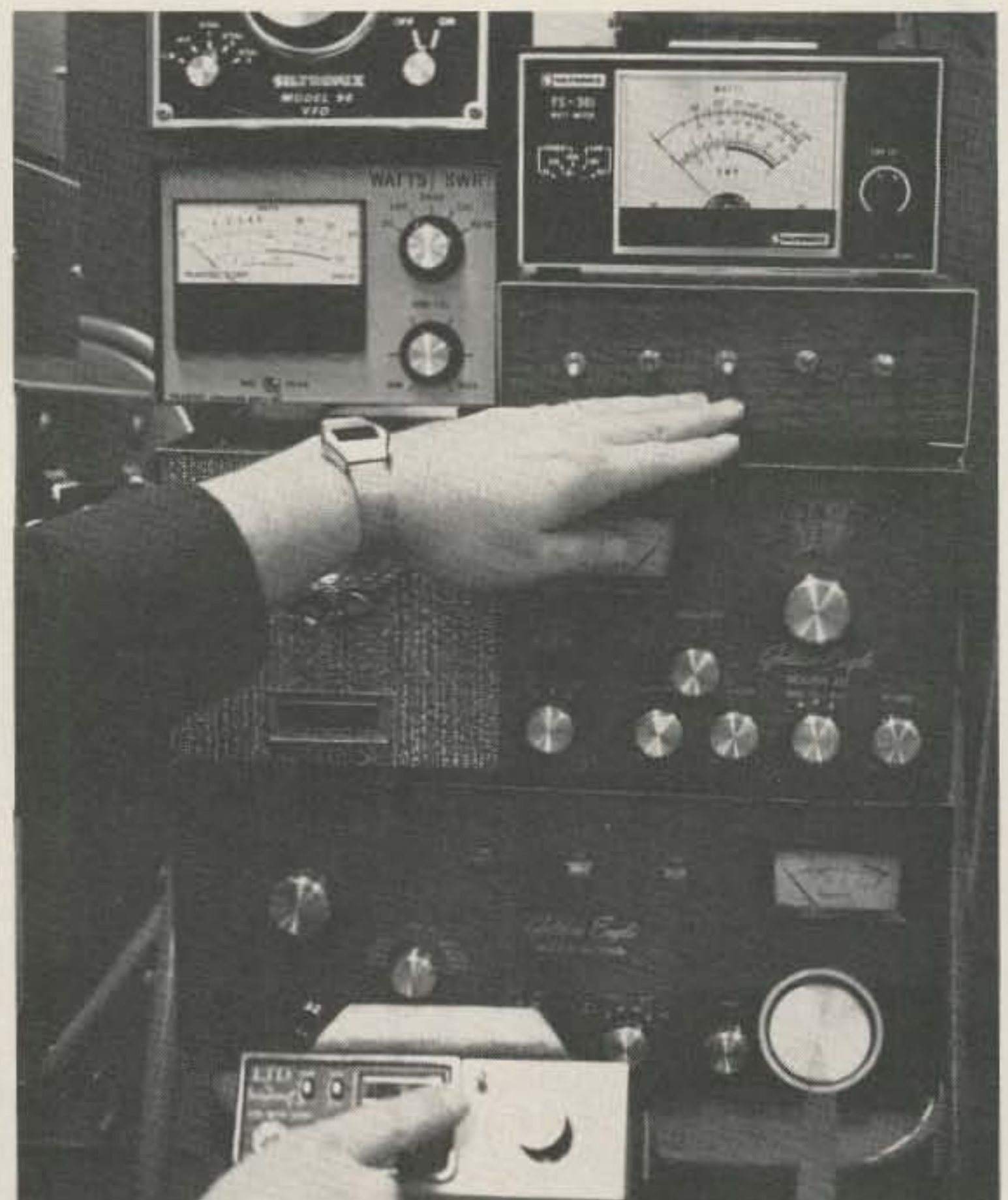
Some of the modified CB gear confiscated in Baltimore-Washington. Note the external switching arrangements which allow out-of-band operation.
