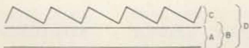
Fig. 1. (a) Reference voltage and regulator output voltage. (b) Minimum ripple voltage. (c) Ripple voltage. (d) Regulator input voltage.
