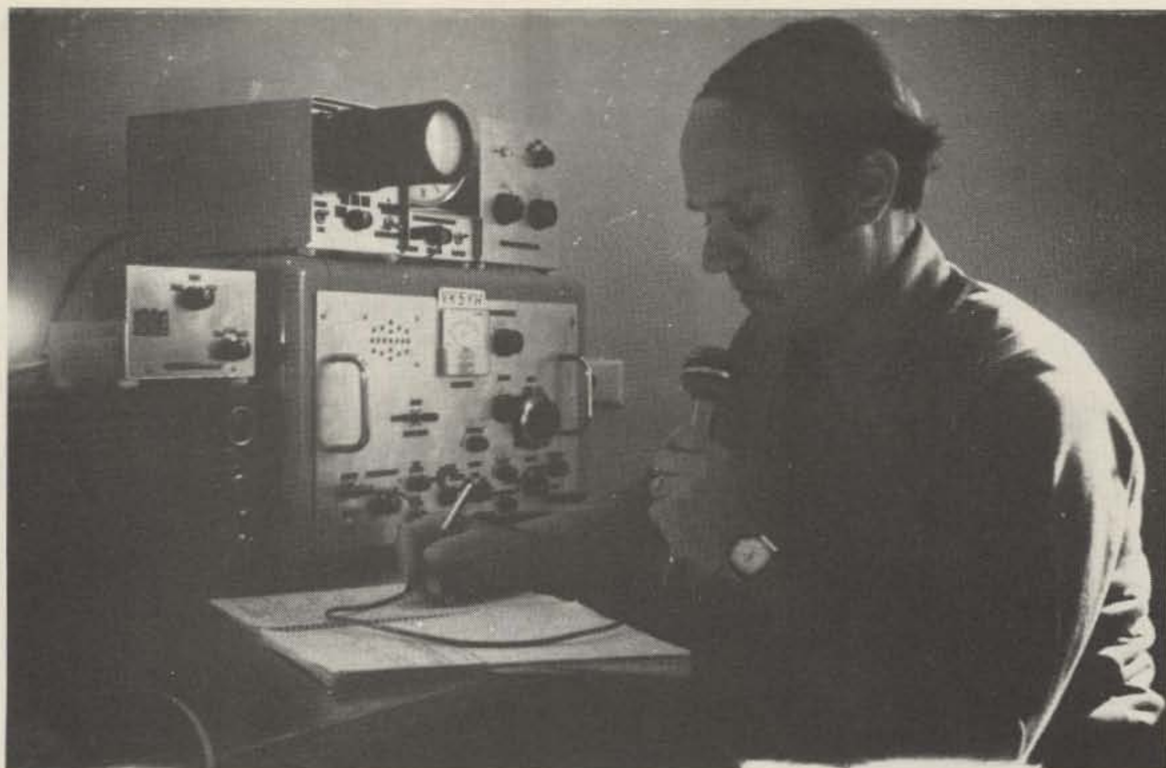
The monitor scope can be seen on top of my allband phasing rig.
