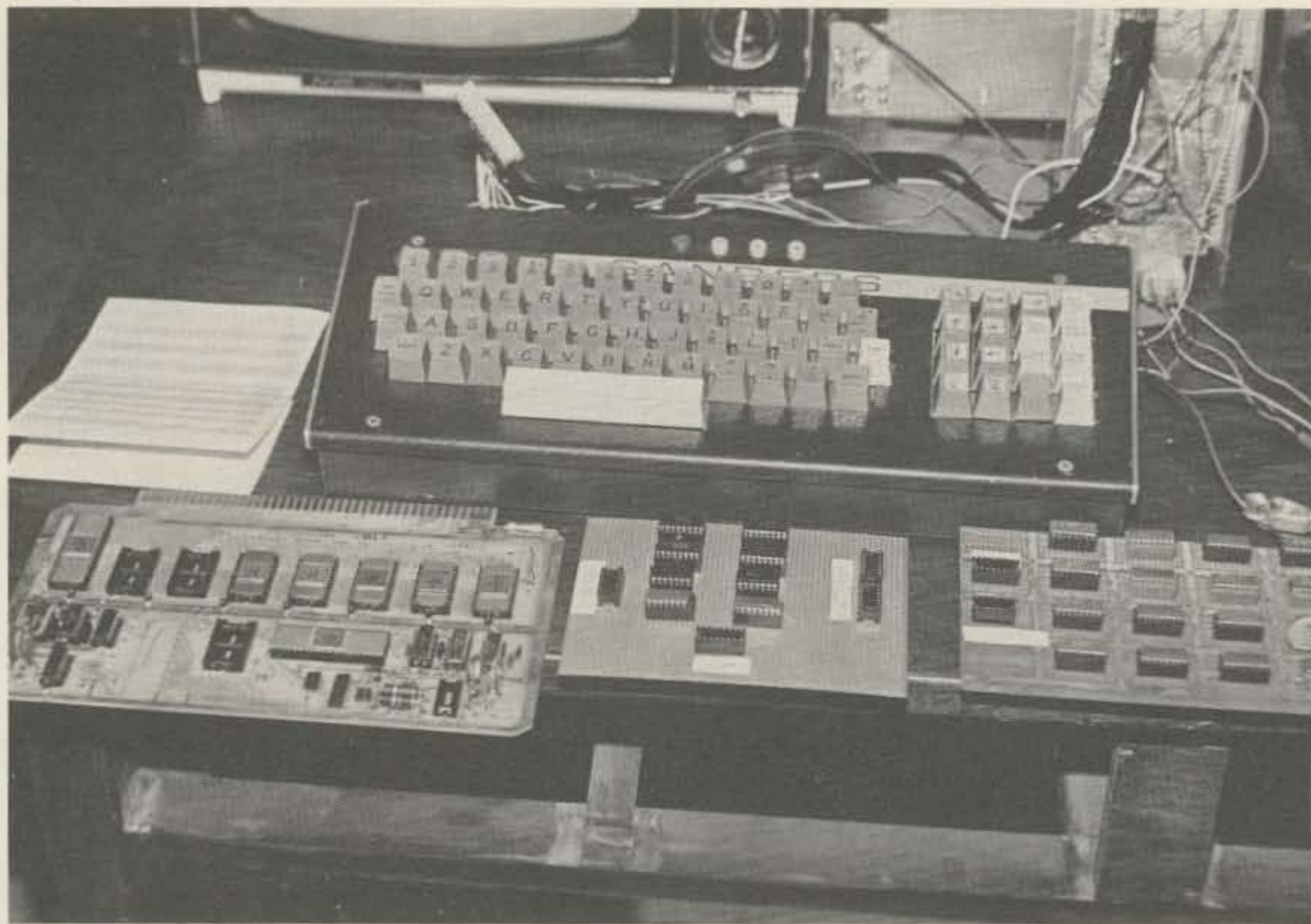
The "Big Three" Motorola MEK 6800 microprocessor evaluation board (left) provides computing power for RTTY system. The memory interface and memory board providing add-on memory capability are alongside. The converted television set in the background provides temporary display capability, while using a Model 19 (not shown) for hard copy. The Sanders 720 ASCII terminal may also be used "on-line" with software ASCII/Baudot conversion.
