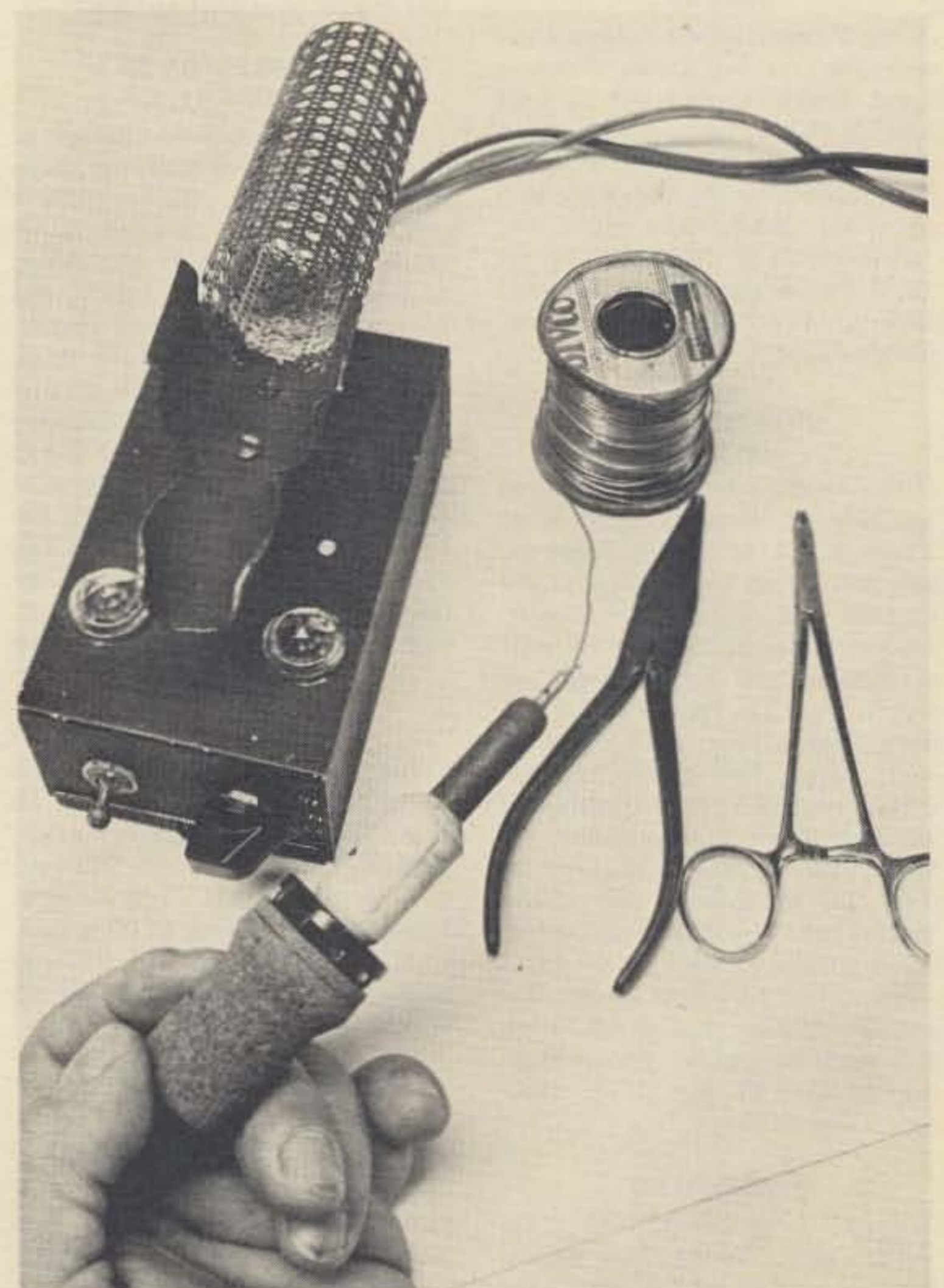
Fig. 1: D1, D2 — 300 V 3A diodes; S1 — SPST toggle switch; S2 — DPDT rotary switch; S3, S4 — SPDT microswitches gang-wired in normal ON position so that weight of iron turns them off.
