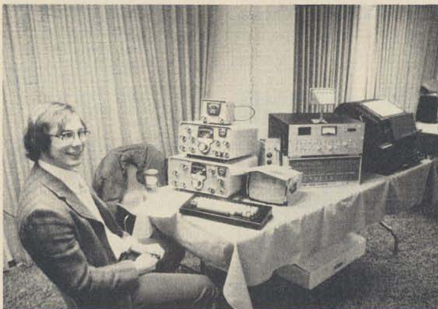
Don Alexander WA8VNP and his RTTY station — winner of the grand prize in the MITS Altair demonstration contest. The home-built system consisted of an Altair 8800 with 8K of memory, an ASCII keyboard, a video display, Baudot teletype and Heath transmitter and receiver. Don also wrote the assembler and editor for the system, as well as the software to run the amateur station. The Altair did the Baudot/ASCII translation, cross-checked calls for duplication, and automatically sent the time and message number along with any text generated by the keyboard. After each contact, a logging entry was made on a model 26 teletypewriter. Don won a complete floppy disk system as the prize.
