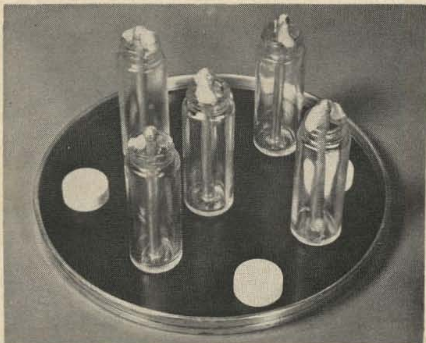
Nine dram bottles used in preparation of large size insulator molding. Greased rod stock, cut to proper length, is held in bottles with modeling clay and an epoxy blob from the bottom. Valspar Casting Resin No. 8880 was then poured in. When dry, glass was cracked off carefully.
