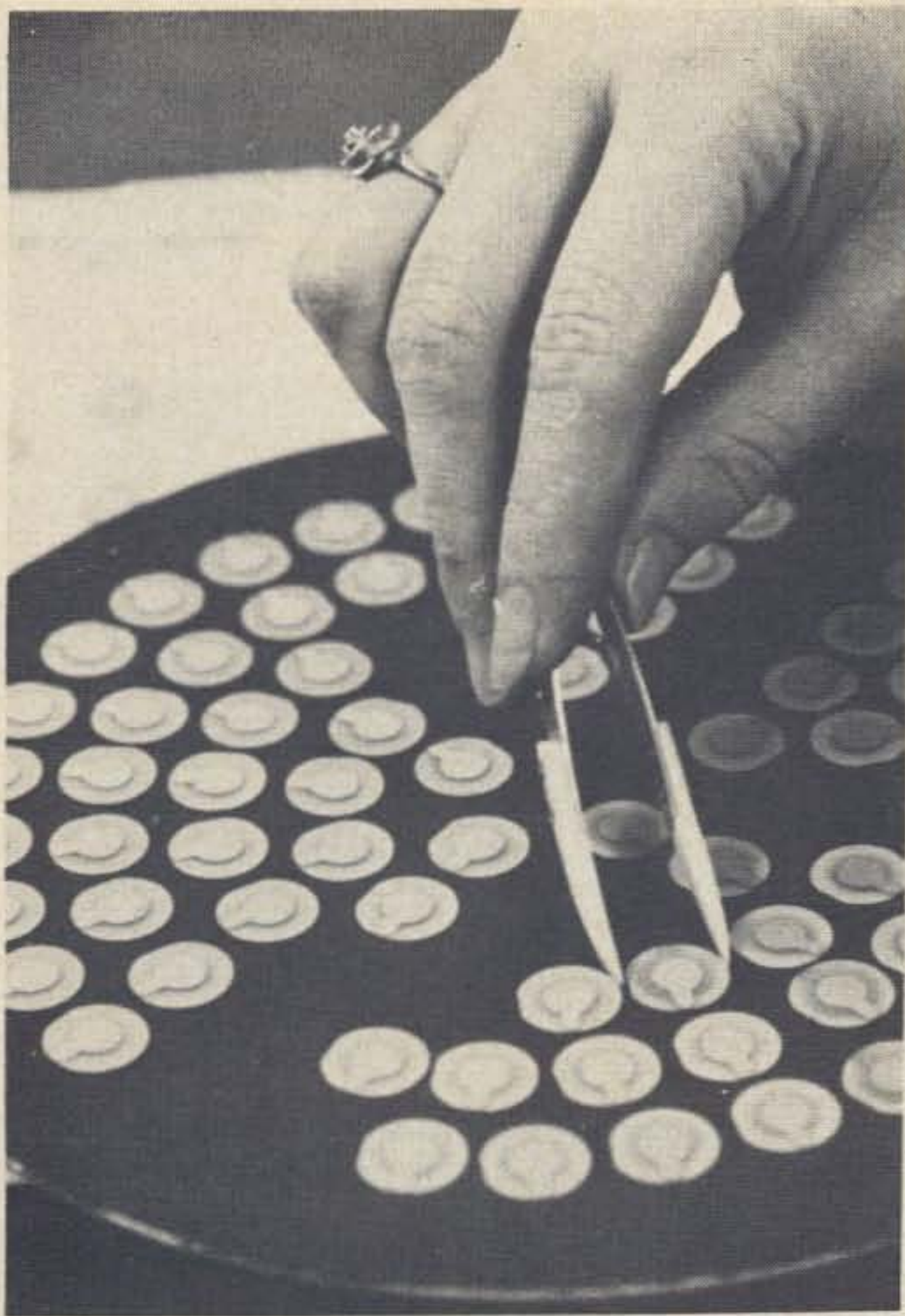
The crystal blanks are put together with electrodes for gold plating.
