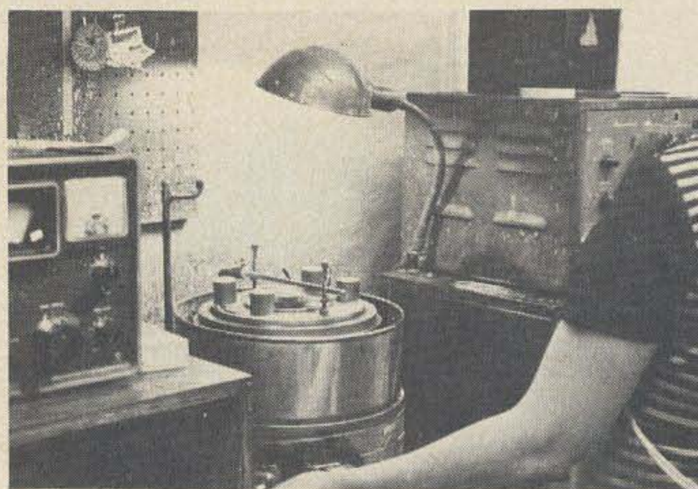
The 129 is at the right and the grinder in the middle — note weights on the crystals to help them grind in.
