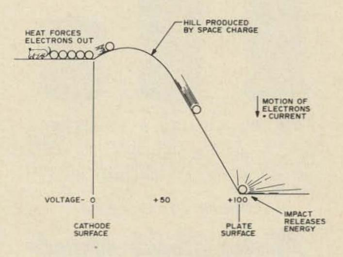
Fig. 2. Action of electrons inside simple diode tube is shown here. Difference in voltage between cathode and plate surfaces forms a "voltage gradient" shown here as a downhill slope. Space charge puts a hump in this hill, near the cathode. Angry ram represents action of heat, boiling electrons off the cathode surface. Those electrons with enough energy to make it over the hump fall down the hill, and hit the plate with a crash, releasing more heat.
