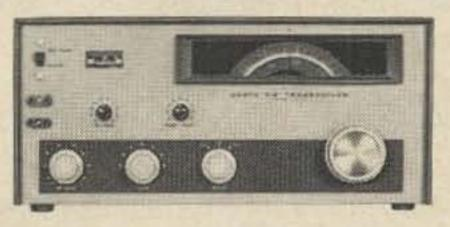
HW-16 Novice CW Transceiver...a high performance 3-band CW transceiver. Covers the lower 250 kHz of 80, 40 & 15 meters. 75 watts input for novice class, 90 watts for general. True break-in CW with solidstate TR switching. Less than 1 uV sensitivity; 500 Hz selectivity with high quality crystal lattice filter. Provisions for VFO transmit with Heathkit HG-10B VFO.
