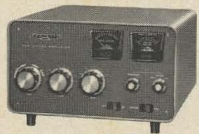
SB-220 2-kW Linear Amplifier...the hottest performing, lowest cost final available. Delivers 2 kW PEP SSB, 1 kW CW & RTTY on the 80 thru 10 meter bands. Built-in solid-state power supply, 120 or 240 VAC. Pre-tuned broadband pi-input for maximum efficiency, low distortion. Two front panel meters for continuous monitoring of plate current, plus switchselected monitoring of grid current, relative power & plate HV.
