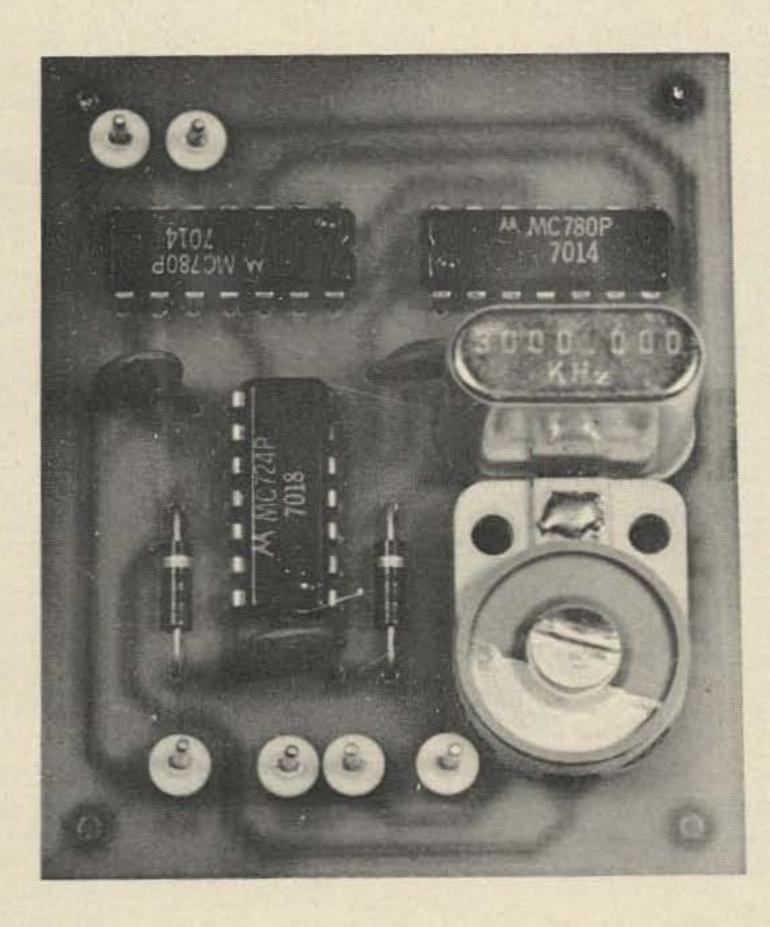
If the .94 in your city seems different from the .94 they have in other parts of the State, you need a standard. The PEP oscillator is that standard...as a single WWV-compared oscillator, it will generate a solid and stable rf signal on all narrowband and wideband channels of the 2 meter band.
