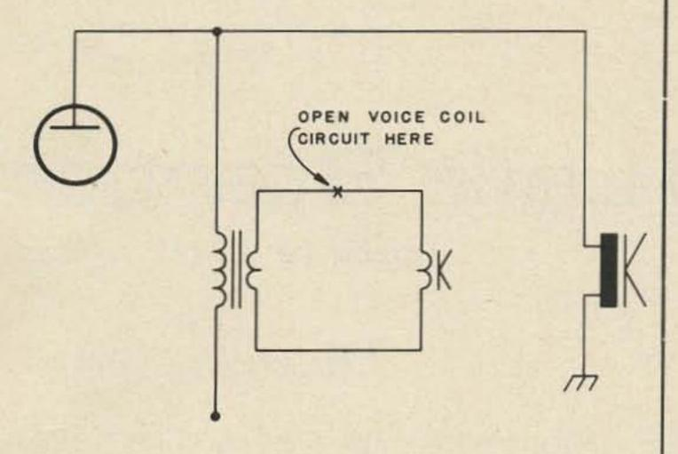
Fig. 1. Method of connecting electrostatic speaker to vacuum tube output.
