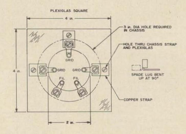
Fig. 2. Layout and plans for the do-it-yourself tube socket.
