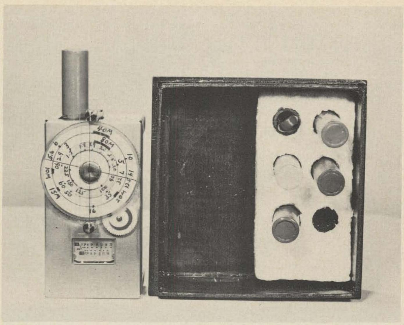
The little gate dipper with spare coils.
