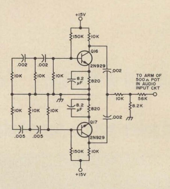
Fig. 8. Two-tone oscillator schematic.
