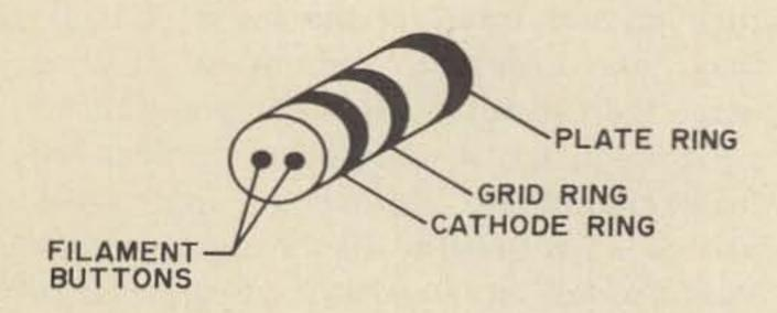
Fig. 6. In quest for UHF operation, tube designers have come up with strange designs. One is this "planar" triode which is made of ceramic, with electrode connections coming out as rings around tube body to eliminate lead inductance as much as possible. Tube operates well into UHF region, but still has an upper frequency limit.
