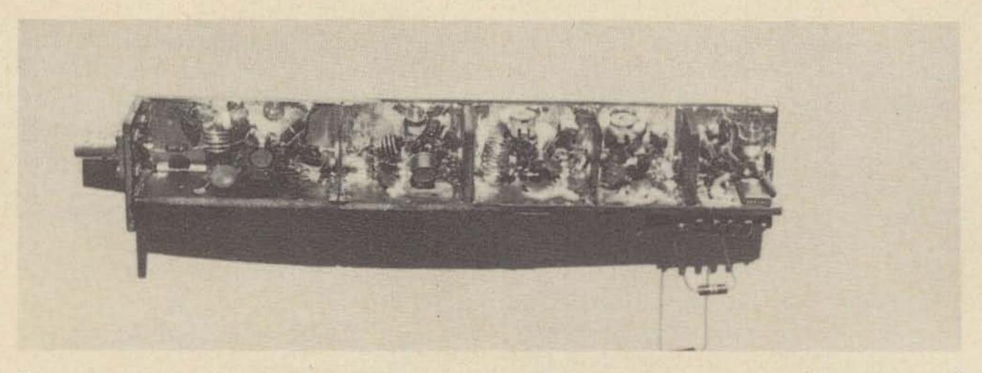
Photograph of the complete minitransmitter strip. Note how stages are shielded into "compartments."
