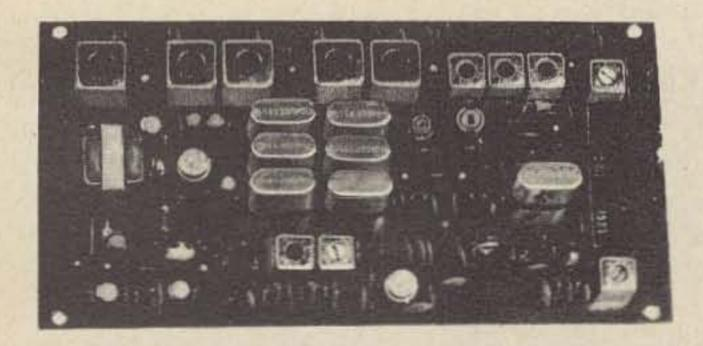
RECEIVER PC BOARD 0.5uv(20db quieting) 94installed 3.5 x 7 x 1 \$ 68.50
