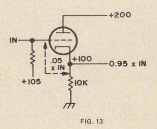
Figs. 10—13. These four schematics illustrate how feedback introduced by resistance in cathode circuit reduces stage gain although tube itself continues to operate unchanged. Voltage applied to grid maintains grid-to-cathode voltage at 5; as cathode voltage changes, grid voltage is changed to always be 5V less.
