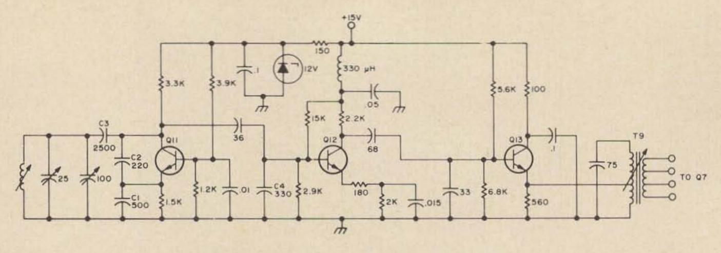
Fig. 7. Variable frequency oscillator (2.9-3.55 kHz).
