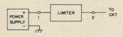
Fig. 2. Block diagram of limiter in typical application.
