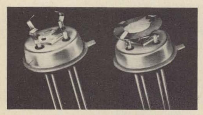
A crystal-controlled microcircuit oscillator (Model MCO-F), which uses thin-film capacitors and resistors on a single substrate, is totally contained within a 4-lead TO-5 Koldweld package. The new unit is designed for application as the local oscillator or second mixer in dual-conversion receivers. It is especially suited for use in advanced paging and personal portable receivers where rugged environmental conditions may be encountered. TRW Electronics, 1100 Glendon Ave., Los Angeles CA 90024.
