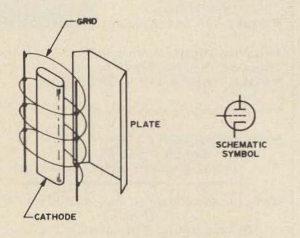
Fig. 4. Introduction of grid between cathode and plate made it possible to control cathode current by means of a separate isolated electrode, and gave birth to electronic amplification as we know it today. Appearance of simple triode is shown at left; schematic symbol is at right.
