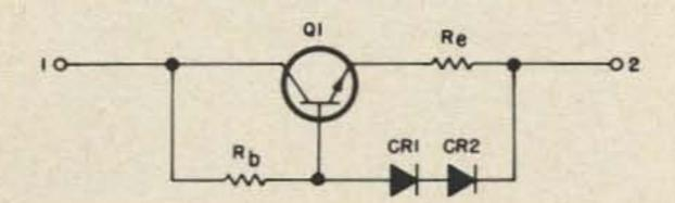
Fig. 1. Series current limiter circuit.
