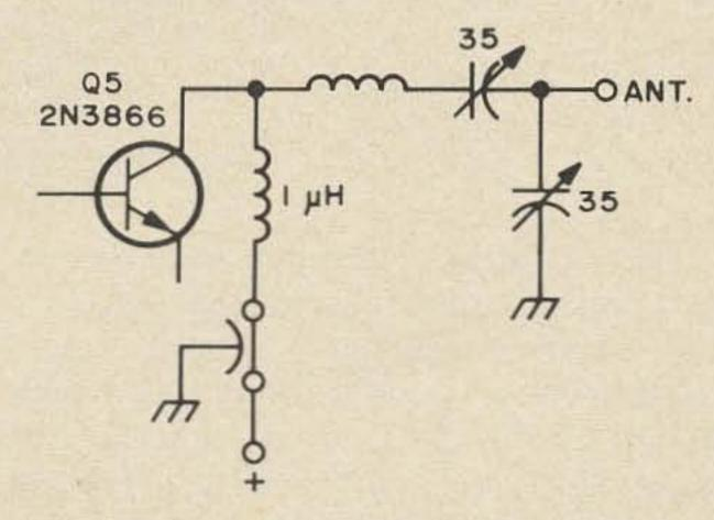
Fig. 2. Alternate Output Circuit. L can be five or six turns 3/8 inch diameter, #18 wire. Try to make it work.
