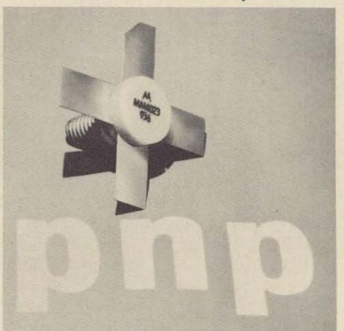
Four new transistors have been added to the industry's only line of silicon PNP rf power devices. The transistors, types MM4020 thru MM4023, bring to nine the number of devices in Motorola's PNP rf power family and increase the variety of output powers available to the designer. These now range from 0.5W to 40W @ 175 MHz.
