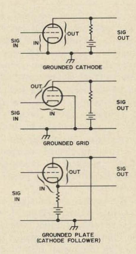
Fig. 9. Differences between the three ways of connecting tubes in amplifier circuits are shown here. These are simplified schematics and leave out all the necessities such as grid bias, coupling capacitors, etc., to emphasize the similarities and differences of the three different circuit types.
