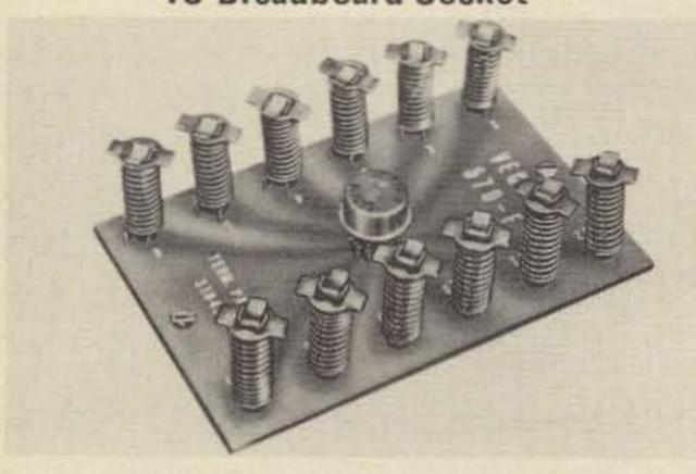
A new device is now available for breadboarding with 12-lead, round TO-5 integrated circuits. The device consists of an epoxy glass wafer, 2-3/8 x 1-5/8 in., on which is mounted a 12-pin socket, the tabs of which have been soldered to two adjacent rows of reliable solderless terminals.
