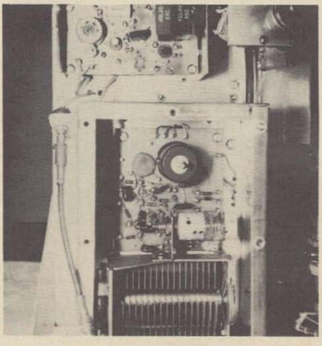
Vfo with lid removed; also shows selectable sideband crystals and balanced modulator.
