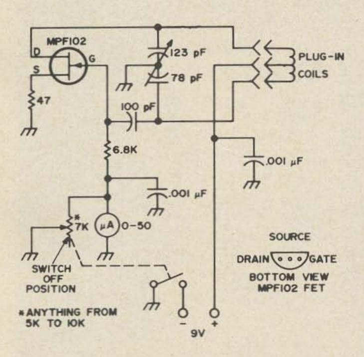
Fig. 1. Schematic diagram of the little gate dipper.
