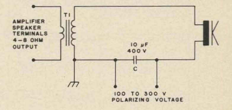
Fig. 2. Method of connecting electrostatic speaker to output of solid state amplifier.
