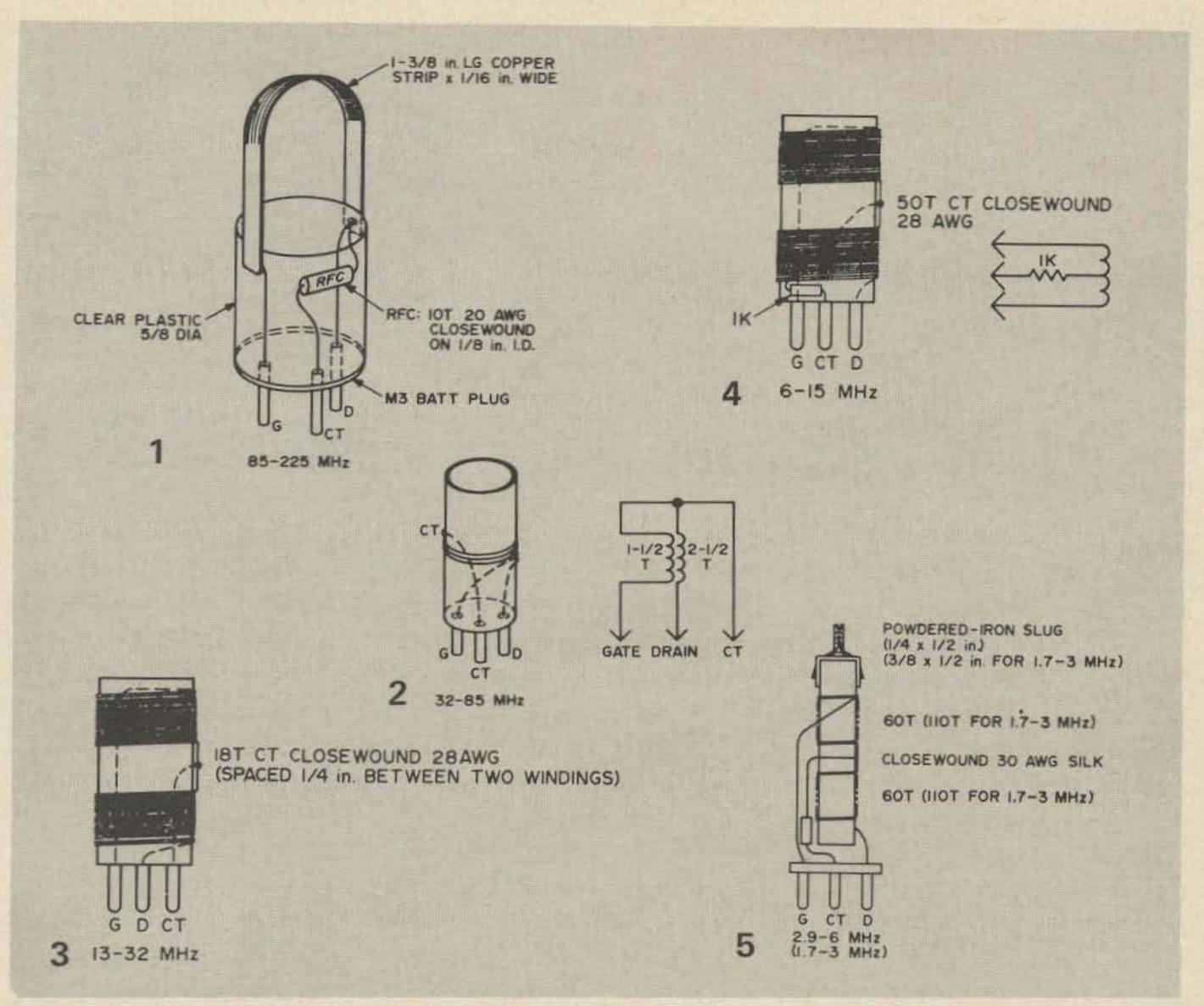
Fig. 2. Coil configurations for various frequencies of resonance.
