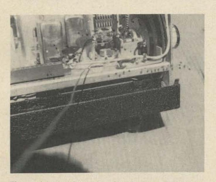
The entire circuit can be placed neatly within the existing space of most transceivers. This photo shows the components mounted near the vfo capacitor in a Galaxy.
