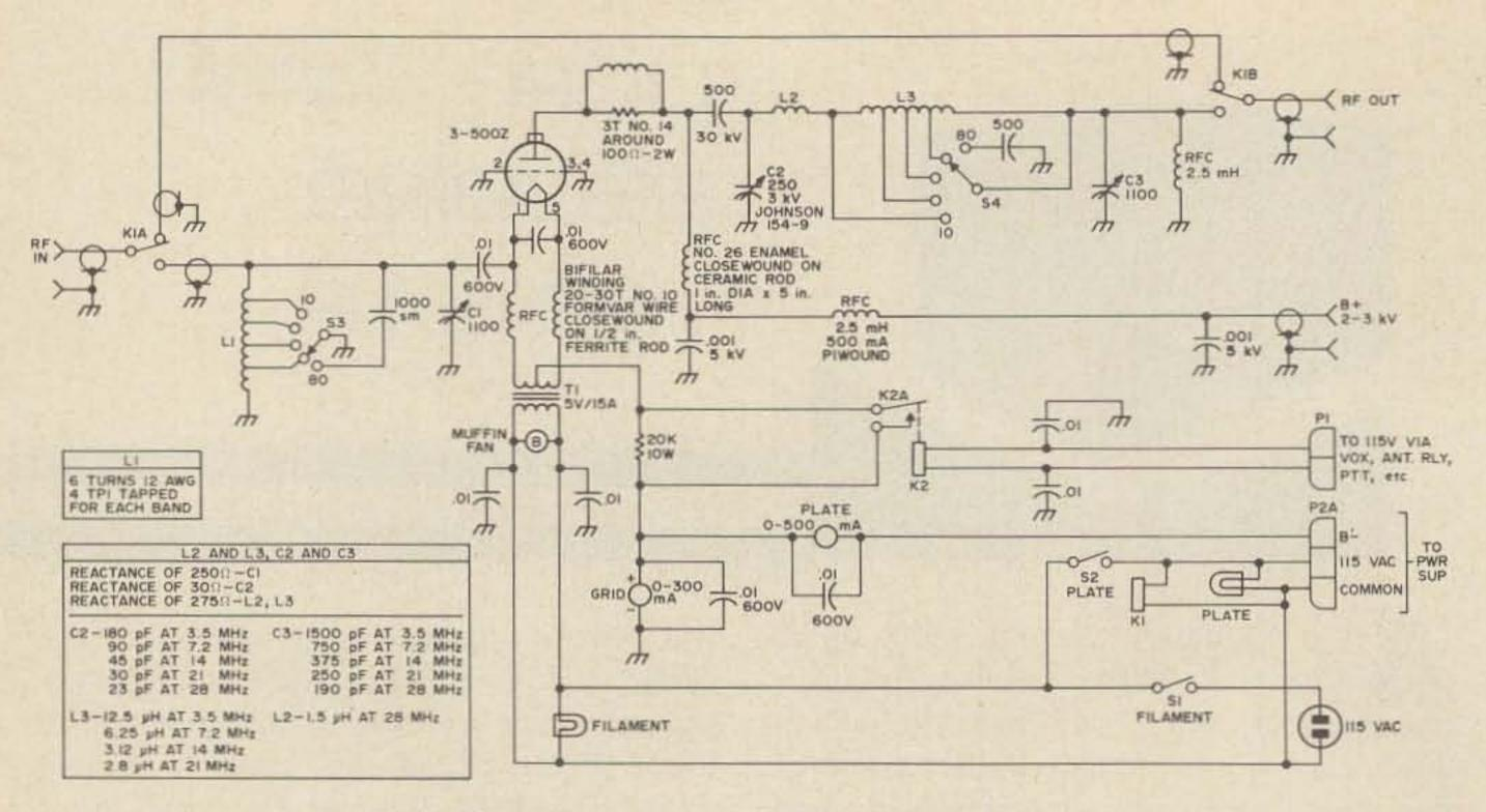
Fig. 1. Schematic of the 3-500Z linear amplifier. Coil data is shown on the table insert.
