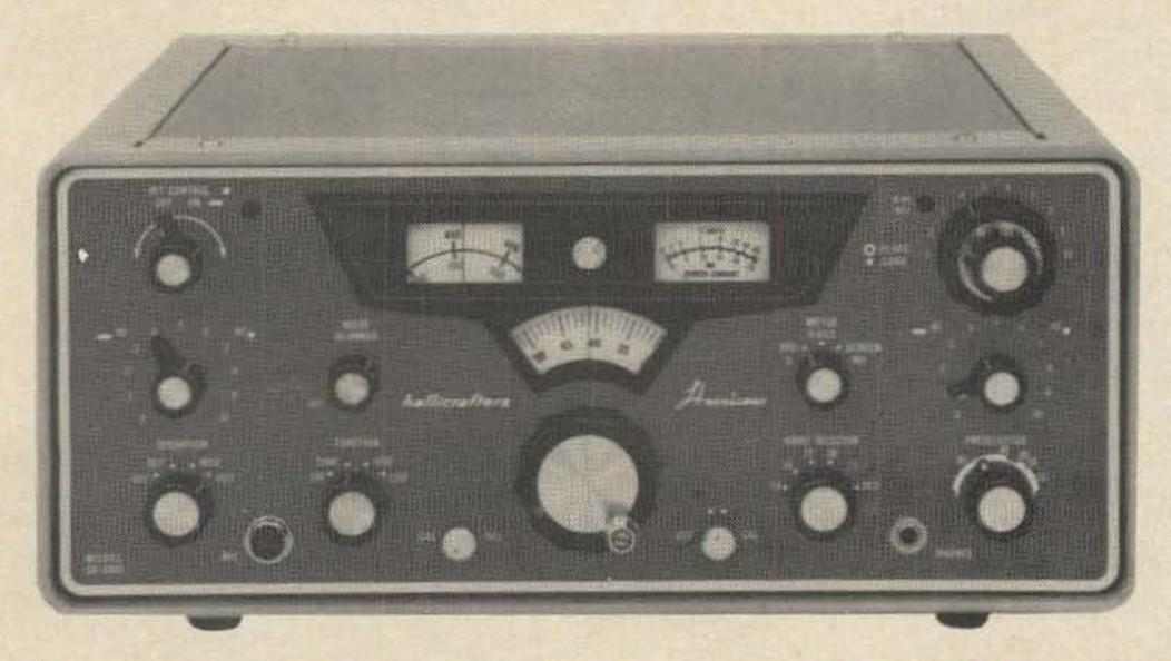
FEATURES: < 1 KC readout • exclusive RIT (Receiver Incremental Tuning) . AALC Amplified Automatic Level Control . built-in Noise Blanker • 100 kHz crystal calibrator, VOX, PTT, Break-in CW < 1 uv sensitivity for 20 db S:</p> N/N • compact rugged cabinet • 2000 watts SSB, 1000 watts CW in a package only 734 x 161/2 x 15 inches . P-2000 AC power supply including built-in speaker, final amplifier plate metering, 110/220 VAC . See WATTS UP at your local Hallicrafters distributor today.
