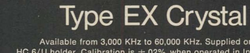
Available from 3,000 KHz to 60,000 KHz. Supplied only in HC 6/U holder. Calibration is ±.02% when operated in International OX circuit or its equivalent. (Specify frequency)
