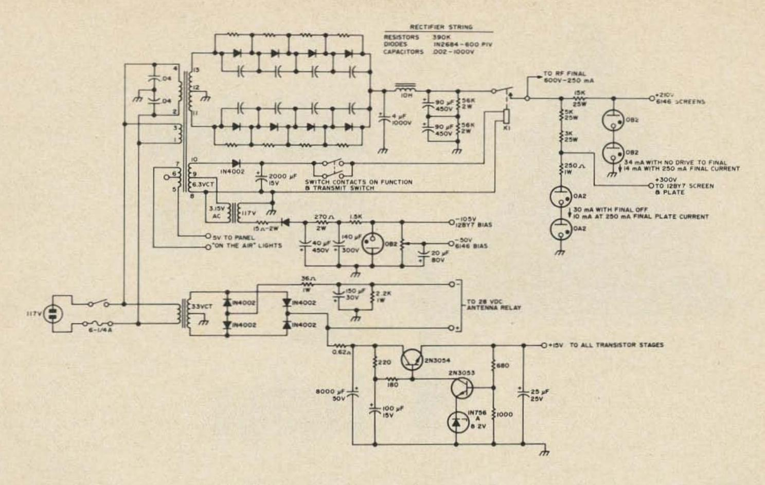
Fig. 9. Power supplies for SSB transmitter.
