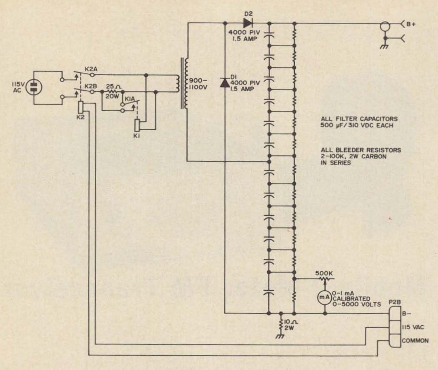
Fig. 3. High voltage power supply.
