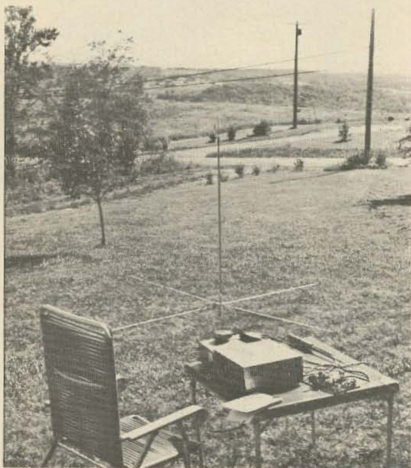
Antenna set up in front yard of author's home for SWR measurements. Additional ground was required for 40-meter operation.
