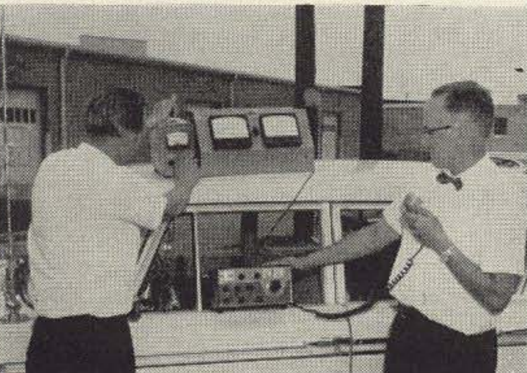
Fred W8FAT checks output of new Drake TR14 transceiver for Clem Wolford W8ENH using a Waters Dummy (no offense) Load Wattmeter.
