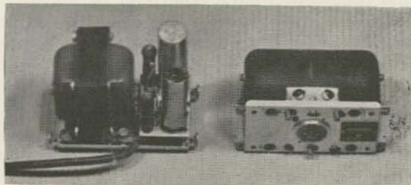
The ac power supply constructed on the original dynamotor plate is shown along with the dynamotor.
