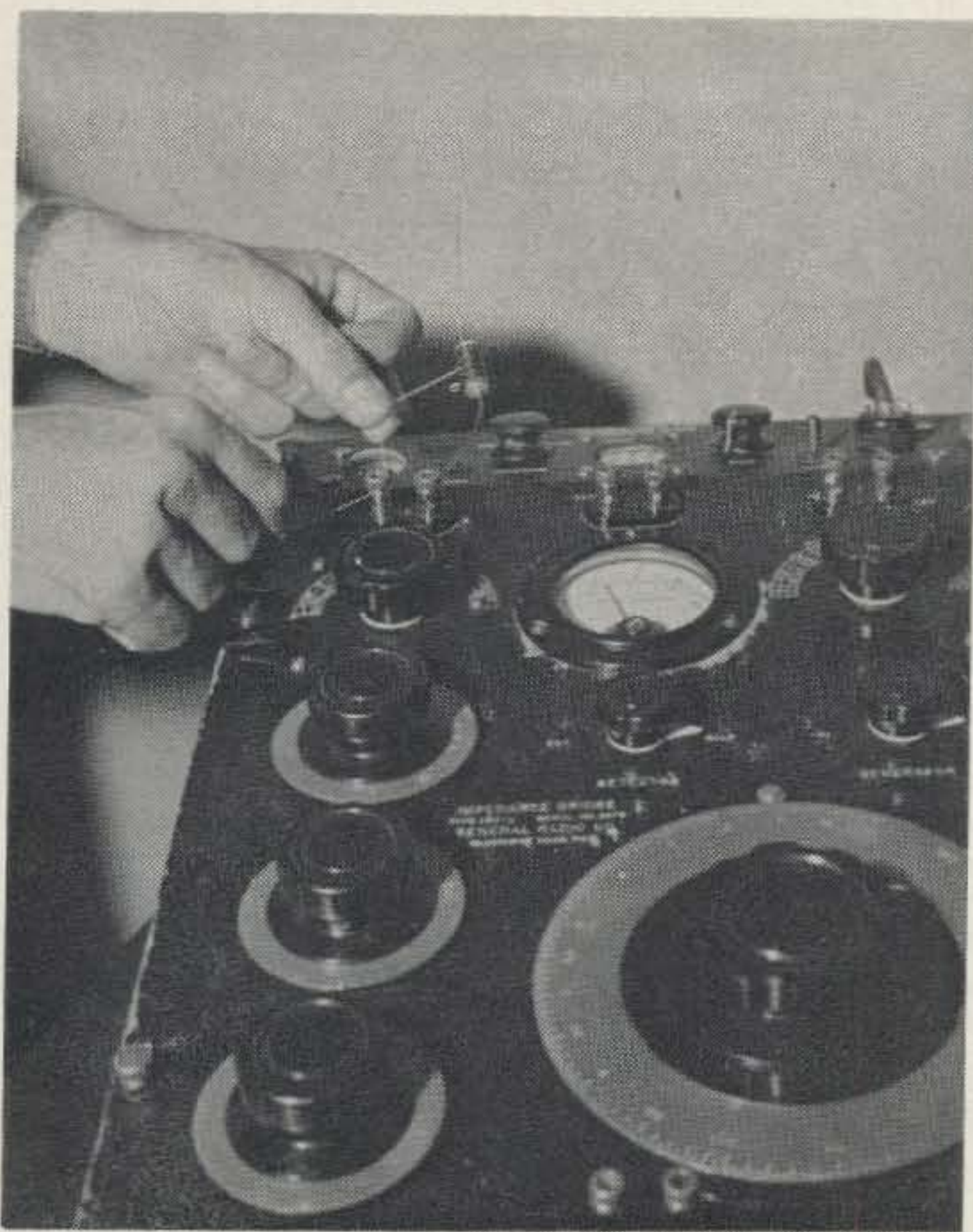
Wire-wound resistors respond to similar treatment. Preset the bridge to the desired resistance value and connect one end of the resistor to the bridge. Unwind resistance wire from the free end of the resistor, passing it through the other terminal of the bridge, until the bridge indicates balance.
