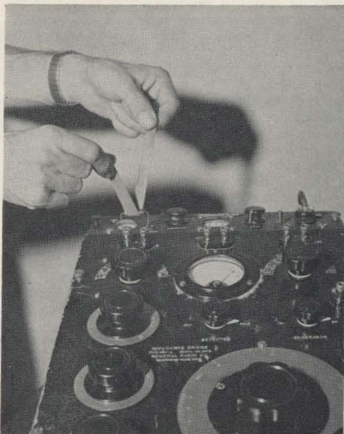
Carbon film resistor is quickly raised to desired value by removing a portion of the carbon film with sandpaper.
