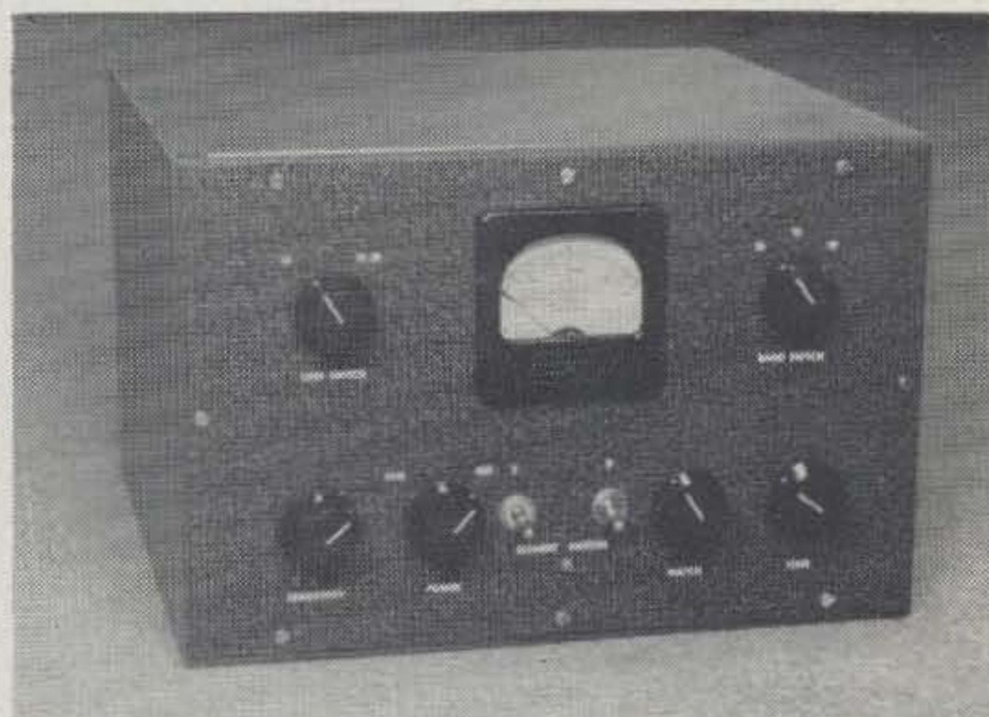
Fig. 6. The antenna tuner, reflected power meter and motor controls are housed in an 8" x 10" x 12" cabinet.
